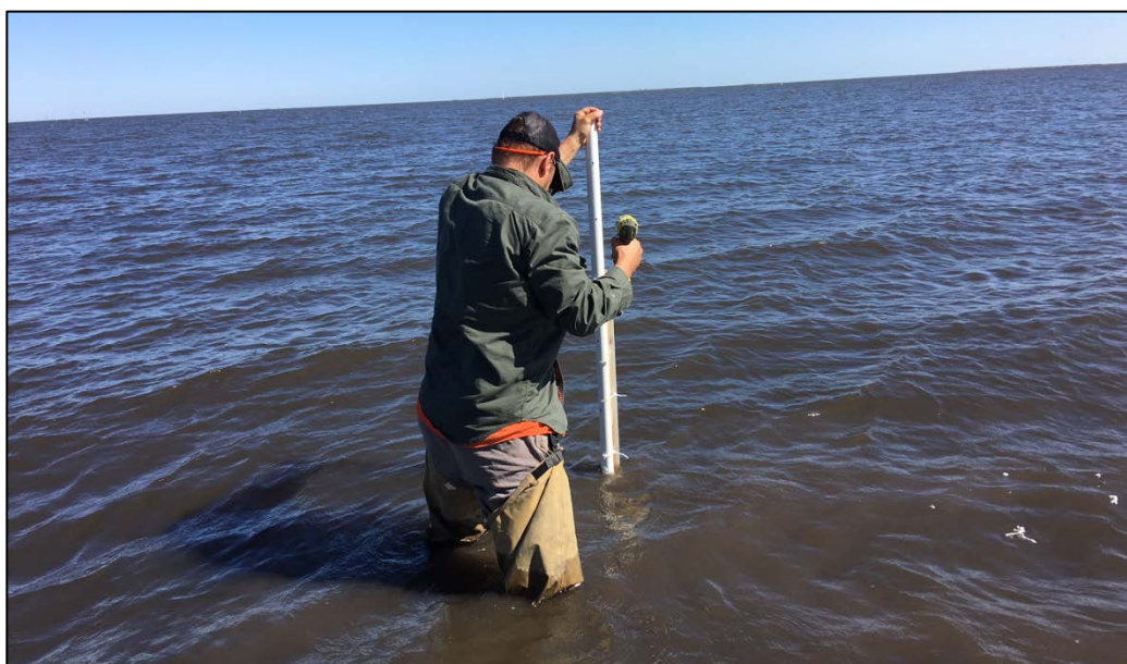
Dr. Lane installing a water level gauge at station C2.
