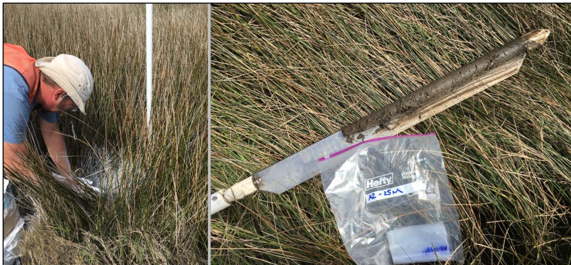
Jason Day deploying feldspar marker horizons (left) and a core for bulk density (right).
