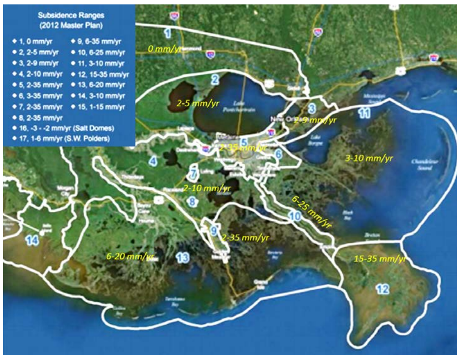
Figure 4-11: Subsidence polygons and estimated ranges of subsidence rates estimated for each polygon in southeast Louisiana as designated for CMP 2012 and left unchanged in CMP 2017 (Reed and Yuill 2017) which governs project development to 2023.
